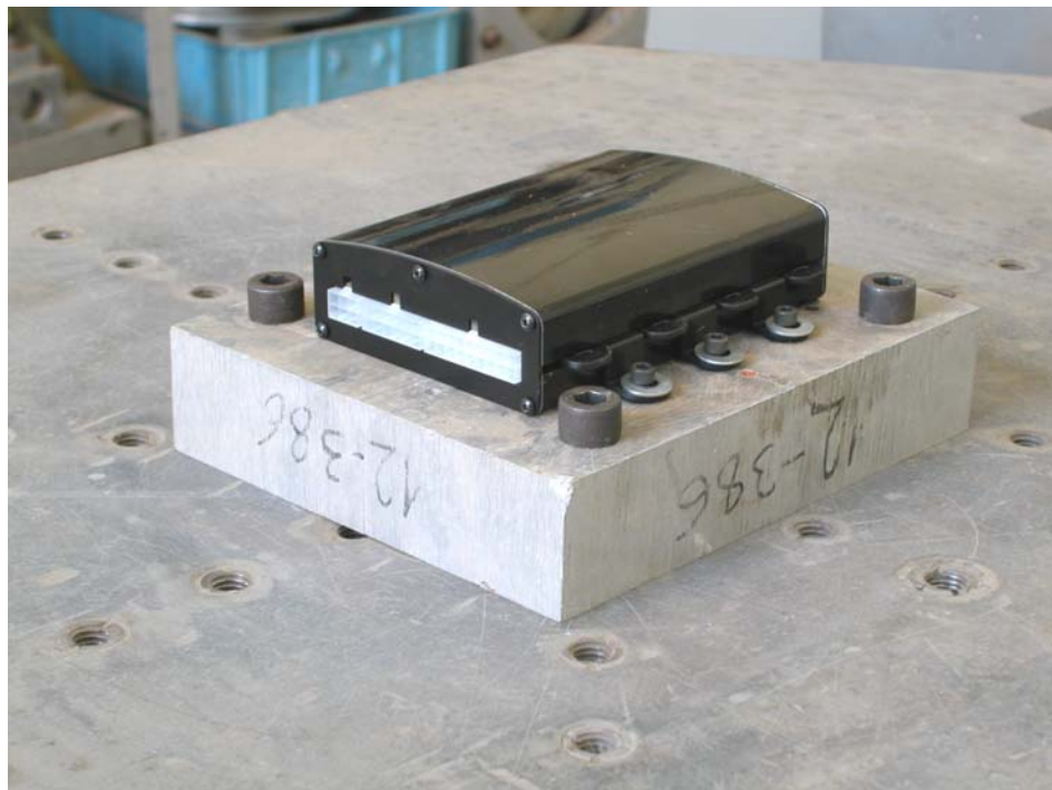
Photo No. 2 : Vibration and Shock testing, Longitudinal axis
