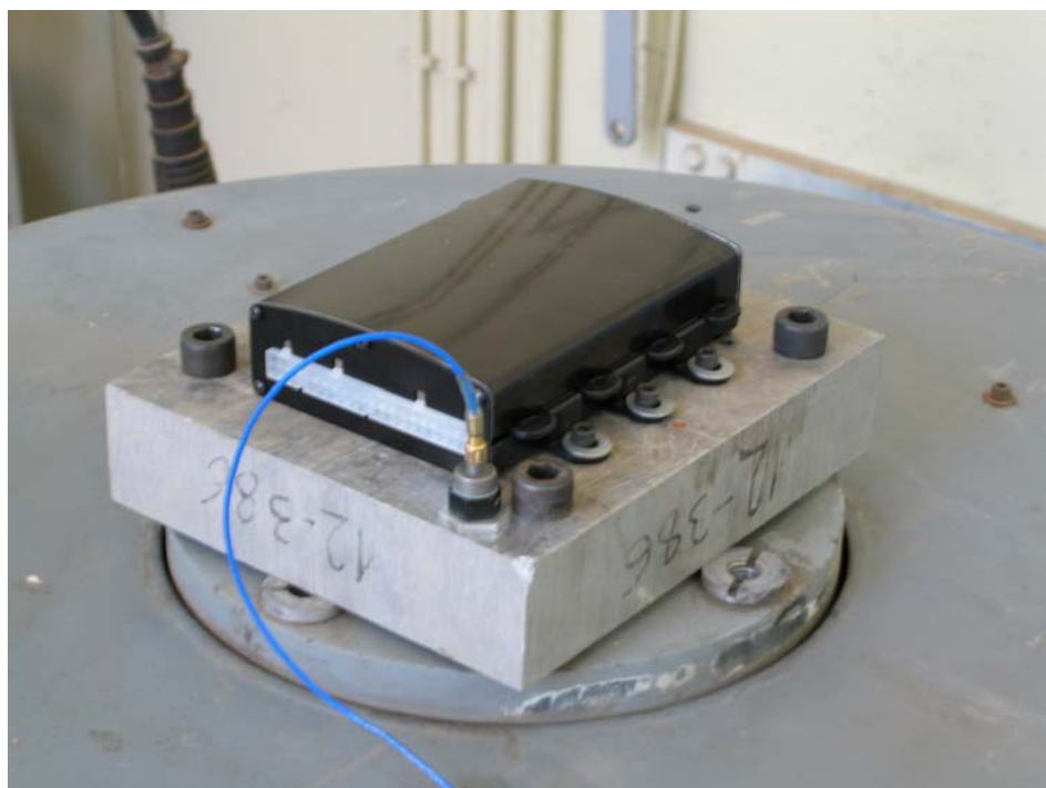
Photo No. 3 : Vibration and shock testing, Vertical axis
